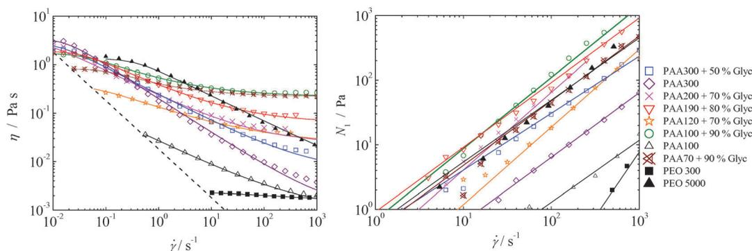
**Fig. 2** Steady shear viscosity and the first normal stress difference as a function of shear rate. The symbols represent the experimental data, the solid lines represent the fits of the White–Metzner model and the dashed line represents  $20\times$  the minimum measurable viscosity, which was calculated based on the minimum torque ( $0.1 \mu\text{Nm}$ ) of the shear rheometer used.
