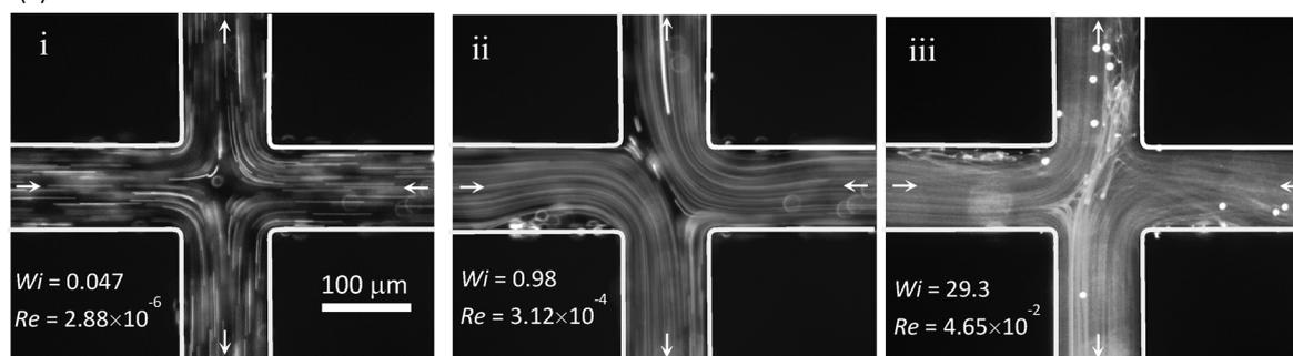
**Fig. 3** Flow patterns in the cross-slot geometry with  $\text{AR} = 1.0$ . (a) Newtonian fluid flow. (b) PAA300 + 50%Glyc viscoelastic fluid: (i) Newtonian-like symmetric flow behaviour, (ii) steady asymmetric flow, and (iii) time-dependent flow (illustrative flow field at a given instant of the oscillation cycle).
