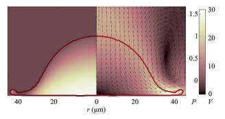
Fig. 5 Simulated droplet impact. Left half: pressure field; the color map indicates the pressure P in  $10^5$  Pa. Right half: velocity field, in which the arrows and the colors respectively indicate the flow direction and flow velocity (in m s<sup>-1</sup>). Simulation parameters:  $D_0=50~\mu m$  and  $V_0=17~m~s^{-1}$ , corresponding to We = 195 and Re = 836. The snapshot is taken at  $t/\tau=0.42$ .
