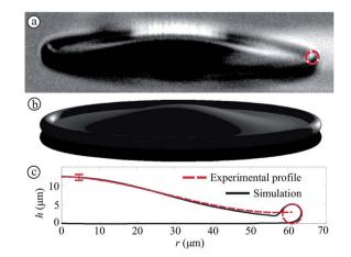
Fig. 8 Bottom view analysis combined with side view and simulation, for the droplet analyzed in Fig. 7. (a) Side view image. In red the rim size is shown, which was used for the analysis of the bottom view images as explained in the main text. (b) Side-view image reconstructed from the fringes in the bottom-view. (c) Rim profiles determined from experiment and simulation. The red vertical line indicates the experimental error.
