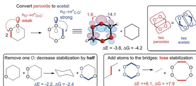
**Scheme 4** Top left: Stabilization energies, orbital interactions, and NBO plots of O1 lone pair,  $\sigma^*_{\text{O2-C3}}$  and  $\sigma^*_{\text{C5-O6}}$  in 1,2,4,5-tetraoxane. Top right: Reactivation of anomeric effect in 1,2,4,5-tetraoxane. Bottom left: Comparison with 1,2,4-trioxane. Bottom right: Comparison with 1,2,5,6-tetraoxacyclooctane. The NBO interaction energies as well as  $\Delta E$  and  $\Delta G$  for the isodesmic reactions are in kcal mol<sup>-1</sup>.
