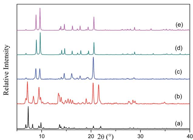
Fig. 1 XRPD patterns of (a) **2fa** simulated from the crystal structure, (b) as-synthesized **2fa** crystals, (c) **2fa** crystals after heating at 120 °C under dynamic vacuum, (d) **3fa** simulated from the crystal structure and (e) **3f** [Zn<sub>2</sub>(ndc)<sub>2</sub>(bpy)] simulated from the crystal structure.
