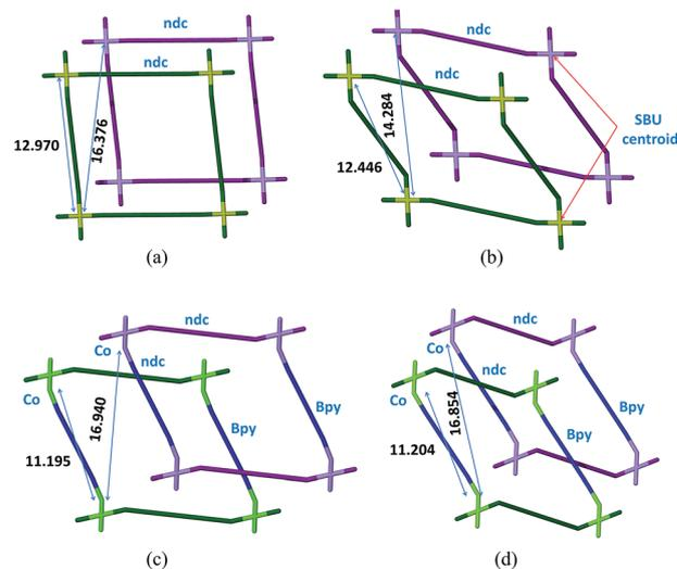
Fig. 5 Schematic representation showing extent of bending and internodal distances for ndc and bpy; (a and b) **2fa** and **2fa'** viewed perpendicular to bpy, respectively and (c and d) **2fa** and **2fa'** viewed perpendicular to ndc, respectively.
