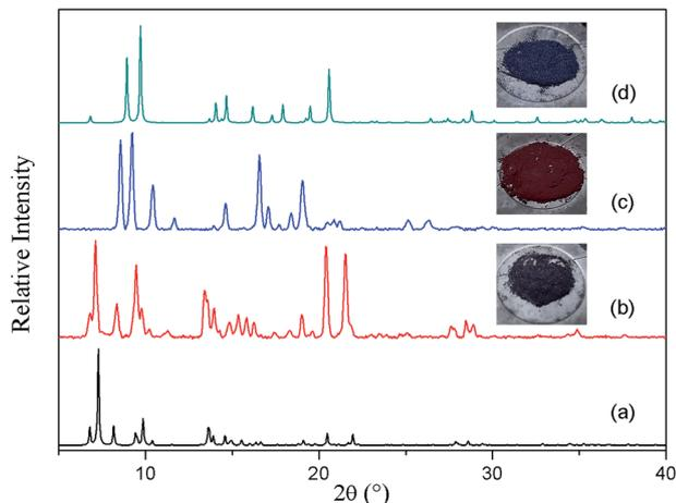
Fig. 2 XRPD patterns of (a) **2fa** simulated from the crystal structure, (b) as-synthesized crystals of **2fa**, (c) **2fa** crystals after heating at 80 °C under dynamic vacuum, (d) **3fa** simulated from the crystal structure.
