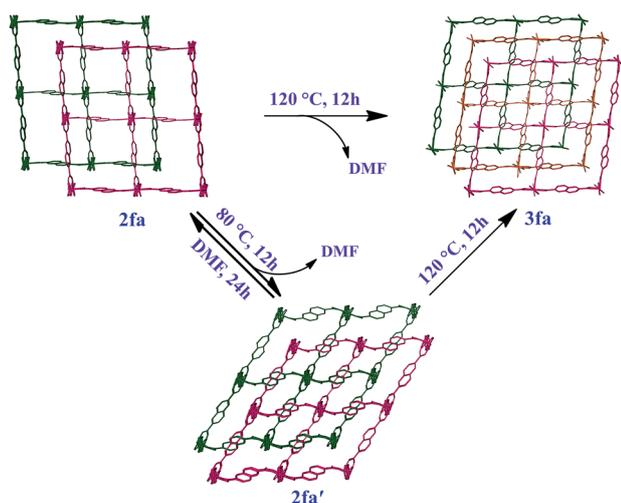
Scheme 1 Schematic representation showing bending and switching of interpenetration in the [Co<sub>2</sub>(ndc)<sub>2</sub>(bpy)] system.
