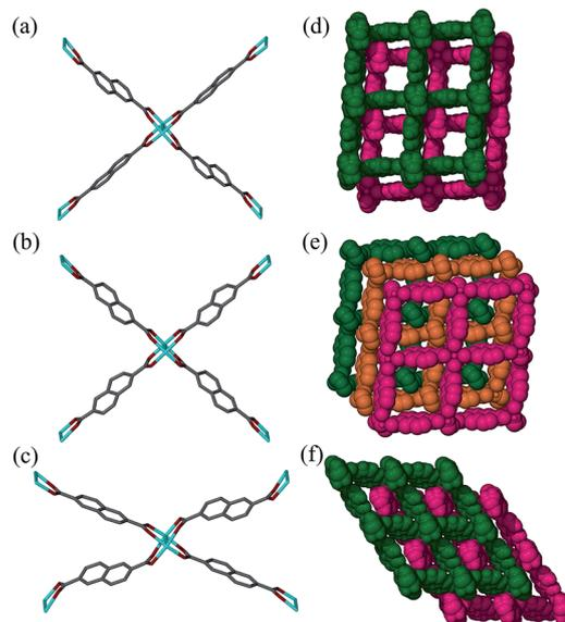
Fig. 3 Perspective view showing  $\text{Co}_2(\text{COO})_4$  paddle-wheel linkages in (a) **2fa**, (b) **3fa** and (c) **2fa'** and packing diagrams of (d) **2fa** (guest molecules omitted), (e) **3fa** and (f) **2fa'**.
