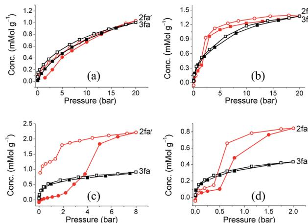
Fig. 6 (a) Methane (b) ethane, (c) propane and (d) butane sorption isotherms of **2fa'** (circles) and **3fa** (squares) at 298 K (shaded and open symbols represent adsorption and desorption, respectively).
