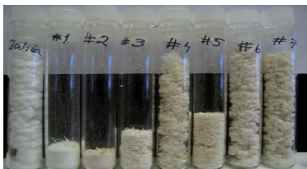
Fig. 6 Appearance of non-milled untreated and in [DBNH][OAc] treated pulp samples.
