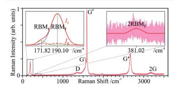
Fig. 8 Raman spectrum after optimal irradiance  $l_1 = 13.24 \text{ kW cm}^{-2}$ The 20-location average (red) has a very low standard deviation (pink). An exposure of other sample regions with this irradiance including previous step-wise exposures produces spectra that fit within this standard deviation. Left inset: the RBM bands vs. those before the laser treatment ( $I_0$ , dashed). Right inset: RBM<sub>2</sub> is so intense that its overtone  $2RBM_2$  is visible.  $R^2 > 0.99$
