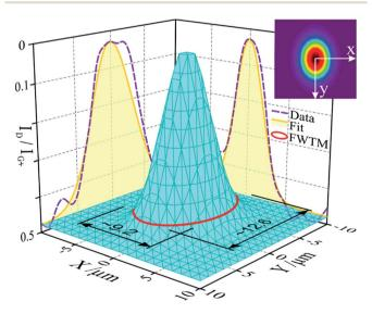
**Fig. 9**  $I_D/I_{G^+}$  over a single, irradiated spot. The asymmetric (slightly elliptic due to beam shape) 3-D Gaussian surface results from the combined parameters of two 2-D Gausses ( $R^2 > 0.98$ ) fitted over b-splined experimental data from intersecting Raman line maps. Note: the vertical axis is inverted to better view the 3-D surface. An average diameter of 10.9 μm (full width at tenth maximum; red ellipse) greatly exceedes the original 2.91 μm beam diameter.
