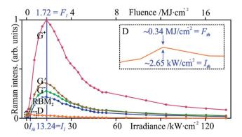
Fig. 4 Peak intensity variations of the studied Raman modes *versus* laser power. All modes peak at  $I_1$  except for D, at  $I_{\rm th}=0.9$  kW m<sup>-2</sup>.
