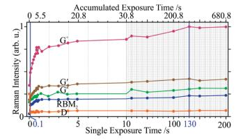
**Fig. 6** Peak intensity variations of the studied Raman modes *vs.* single and accumulated (nonlinear) exposure times. The D mode saturates abruptly after a 0.1 s shot, while the other modes need 130 s to do so. The time scale proportionality is stretched in the first ten seconds to show more detail.
