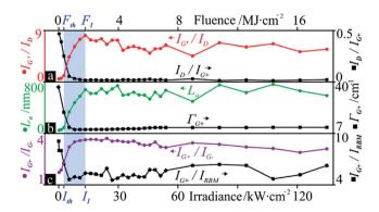
Fig. 5 From top to bottom, all *versus* irradiance and fluence: Raman purity (normalized  $I_{G'}/I_D$ ) and quality ( $I_D/I_{G^+}$ ) indicators (a); inter-defect distance ( $L_a$ ) and full width at half maximum of  $G^+$  ( $\Gamma_{G^+}$ ) (b);  $G^+$  vs.  $G^-$  growth, *i.e.* G mode splitting gap ( $I_{G^+}/I_{G^-}$ ), and  $G^+$  vs. RBM growth, *i.e.* gap between the two main order-induced peaks ( $I_{G^+}/I_{RBM2}$ ) (c).
