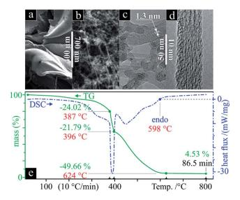
Fig. 1 SEM (a and b), TEM (c and d), TGA and DSC (d) of the pristine SWCNTs.
