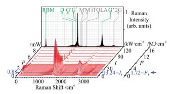
Fig. 3 Power sweep: Raman signal vs. power (P), power density (I) and fluence (F). A sharp non-proportional increase in the intensity of the graphitic order-induced RBM, G and G' modes is observed up to 0.88 mW (blue spectrum, marked by arrow), followed by a gradual signal intensity drop. Peaks are labelled (green & underlined, for those used in this study) on the rear plane containing the accumulated shadows of all spectra.
