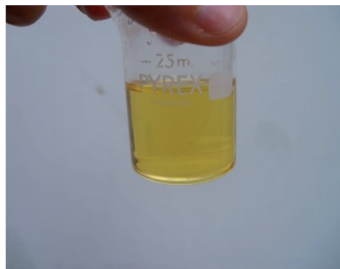
Fig. 4 Photo of T20BD + 5% ECPOSS mixture after ultrasonication and 1 h in a stirred oil bath at 120 °C.
