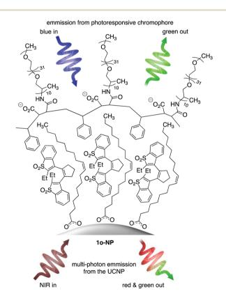
Fig. 1 The self-assembled nano-system (1o-NP) containing the amphiphilic polymer wrapped around the lanthanide-doped upconverting nanoparticles with encapsulated diarylethene chromophores. The green emission from the organic chromophore is turned 'on' using UV light to ring-close the diarylethene. The multiphoton emission from the UCNPs is always on when irradiated with NIR light.
