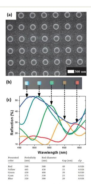
**Fig. 1** (a) Scanning electron microscope (SEM) image of the top view of Ag vertical nanorod arrays on a quartz substrate with a periodicity  $p=550\,$  nm. (b) Optical image of the reflective colors from different Ag nanorod arrays. (c) Measured reflection spectra of the corresponding arrays as a function of wavelengths. The table below (c) shows the size parameters of nanostructures for different colors in (b) and (c). Reproduced with permission.  $^{50}$  Copyright 2013, RSC.
