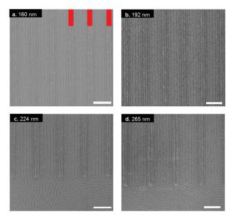
Fig. 2 Top-down SEM images of graphoepitaxially aligned porous PS-b-P4VP templates in HSQ gratings following swelling of P4VP domains using ethanol vapor. (a)—(d) Show alignment of PS-b-P4VP features in 50 nm HSQ gratings (red bars in image a) at channel widths of (a) 160 nm, (b) 192 nm, (c) 224 nm and (d) 265 nm. (c) and (d) Show areas where alignment has taken place from open areas in to the HSQ trench gratings. Scale bars are 200 nm.
