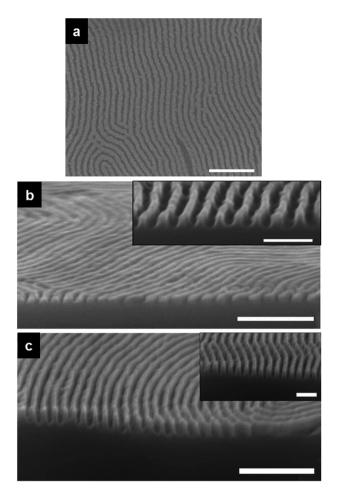
Fig. 6 (a) Top-down SEM of Si nanofins following plasma etching of Fe<sub>2</sub>O<sub>4</sub> nanowire hardmask for 1 minute and 30 seconds (b) Crosssection SEM image of sample (a) while (c) shows cross-section SEM image of an Fe<sub>3</sub>O<sub>4</sub> nanowire hardmask plasma etched for 2 minutes. Insets in (b) and (c) show highly defined uniform nanofin arrays. Main scale bars are 250 nm while inset scale bars represent 100 nm.
