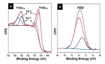
Fig. 5 (a) High resolution XPS spectra of Fe 2p core level of iron oxide (Fe $_3$ O $_4$ ) nanowires following UV/O $_3$  treatment. (b) High resolution XPS spectra of Al 2p core level of aluminium oxide nanowires ( $_7$ -Al $_2$ O $_3$ ) following UV/O $_3$  treatment. Survey spectra and high resolution O 1s core level spectra are shown in ESI Fig. 21 and 22† for both samples.
