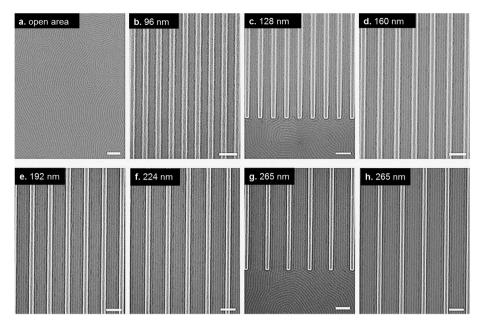
Fig. 4 (a) Shows top-down SEM image of  $\gamma$ -Al<sub>2</sub>O<sub>3</sub> nanowires in open area of HSQ substrate. (b)–(h) Top-down SEM images of aligned  $\gamma$ -Al<sub>2</sub>O<sub>3</sub> nanowires in 50 nm HSQ gratings with channel widths indicated in image. All scale bars are 200 nm.
