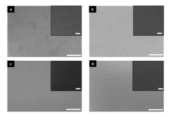
Fig. 1 PS-b-P4VP BCP films were spin coated from a 0.5 wt% solution on to acetone degreased Si substrates. Top-down SEM images are shown in (a)–(d) after solvent vapor annealing with chloroform at room temperature (~290 K) of a 24 nm thick PS-b-P4VP BCP film for (a) 30 minutes, (b) 1 hour, (c) 2 hour and (d) 3 hours respectively. Note films were exposed to ethanol vapors following solvent vapor annealing to create porous structures. Scale bars are 500 nm, while inset scale bars are 100 nm.
