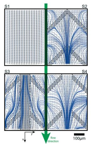
Fig. 5 Vector maps and corresponding streamlines. Visualization of the time-averaged flow profile (velocity vectors: black arrows, streamlines: blue lines) at Re = 400 for the different flow promoter designs.
