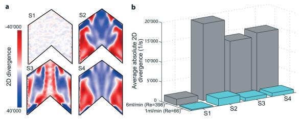
Fig. 4 Fluid dynamically induced mixing propensity. (a) 2D divergence maps derived from μPIV experiments highlighting the generated gradients in the out-of-plane component of the velocity vector for samples S1-S4. (b) Average absolute divergence  $|\operatorname{div}_{2D}|$  for the different designs and
