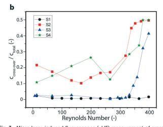
Fig. 3 Micro laser-induced fluorescence (µLIF) measurement of crossover. (a) Illustration of measurement principle and typical images obtained for situations with (image to the right) and without advective cross-over (image to the left). (b) Ratio of the cross-over concentration of the dye Rhodamine B to the total concentration. Values of 0.5 indicate total transversal mixing.
