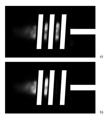
Fig. 3 Effect of methanol on plasma volume. (a) Introduction of 3% v/v HNO<sub>3</sub>; (b) introduction of 10% (m/m) methanol. The positions of the three turns of the load coil and the injector are represented with white bars for clarity. Both images were recorded under identical photographic conditions (aperture setting, exposure time). Note that in image (b) the plasma withdrew from the space between the first and the second turn of the load coil.
