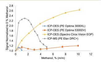
Fig. 1 Effect of increasing methanol concentration on the signal of Se in ICP-OES (Se 203.985 nm) and ICP-MS (m/z = 78) recorded on different instruments. The Se concentration was 10 mg  $L^{-1}$  in ICP-OES and 10  $\mu$ g L $^{-1}$  in ICP-MS. No internal standard was used; the Einzellens of the ICP-MS was tuned for aqueous solutions. Error bars: standard deviation, n = 5
