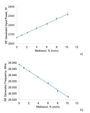
Fig. 2 Power drawn by the RF generator for a nominal output of 1350 W (a) and frequency response of the generator (b) as a function of the methanol concentration nebulized during measurement. The error bars represent the standard deviation of five independent experiments.
