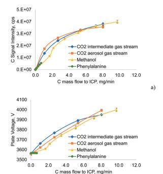
Fig. 4 Signal intensity of the C I 193.091 nm emission line and power vacuum tube plate voltage as a function of the carbon mass flow introduced into the ICP for the investigated carbon sources. The error bars represent the standard deviation of five independent experiments.
