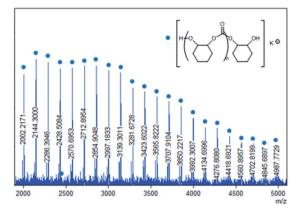
Fig. 3 MALDI-ToF spectrum of the low  $M_n$  fraction of PC (Table 1 entry 2), a single series is observed corresponding to:  $[HO(C_7H_{10}O_3)_nC_6H_{11}O_2]K^+ = [(142.15)_n + 116.16 + 39.1].$
