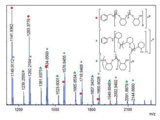
Fig. 7 MALDI-ToF spectrum of the PCHC obtained in Table 3 entry 7, using 20 equiv. of H<sub>2</sub>NBn.
