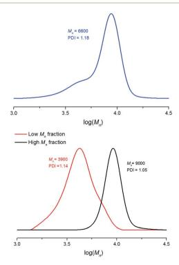
Fig. 2 Top: molecular weight distribution of the isolated (crude) PCHC polymer (Table 1 entry 2) and bottom: the separation of PCHC into two fractions of low and high  $M_{\rm w}$ .
