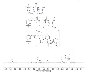
$^{1}$ H NMR spectrum (400.0 MHz, CDCl<sub>3</sub>- $d_{1}$ , 298 K) of the isolated PCHC produced in the polymerization with H<sub>2</sub>NBn additive (Table 3, entry 7). The asterisk denotes the residual protio-solvent.
