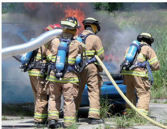
Fig. 2 Fire crew tackling an engine compartment fire (1994 Ford Aerostar minivan) during knockdown on vehicle 1. Flexible metallic sampling duct held by a member of the fire crew, close to the nozzle operator's shoulder.
