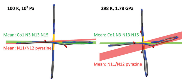
Fig. 3 Perspective view of [\text{Co}^{\text{II}}(\text{dpzca})_2] at 100 K and atmospheric pressure (left) and at 293 K and 1.78(9) GPa (right) highlighting the twisting of the N11/N12 pyrazine ring: In order to minimise the volume of the complex, whilst maintaining the elongation in the second ligand strand, one of the pyrazine rings on the second ligand strand [the N11/N12 ring], has shifted significantly further out of the plane defined by the Co(1) centre, the other two donors on the same ligand strand [N(13) and N(15)], and the imide nitrogen [N(3)] on the other ligand strand. The mean plane of the N11/N12 pyrazine ring is at an angle of 16.9^\circ to that plane in the 1.8 GPa LS structure, compared to just 3.3^\circ in the low temperature LS structure. This also distorts the octahedron significantly (Table 1), which is best identified by looking at the \sum_4 , rather than the \sum_{12} where the effect is diluted by the other (relatively unchanged) cis angles, and even more clearly by the tetragonality factor T which shows maximum axial elongation of the octahedron at 1.78 GPa, consistent with this being fully LS, hence showing maximum Jahn Teller distortion.
