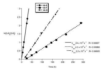
Fig. 9 Plot of  $ln([LA]_0/[LA]_t)$  vs. time of initiator Al-E, F and G. Conditions: [LA]<sub>0</sub> = 1 M, 1:1:100 [I]: [iPrOH]: [LA], toluene, 348 K.
