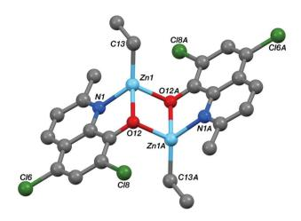
Fig. 6 The crystal structure of the C<sub>i</sub>-symmetric complex Zn-A. Selected bond lengths (Å) and angles (°); Zn1-N1 2.0866(17), Zn1-O12 2.0776(14), Zn1-C13 1.984(2), Zn1-O12A 2.0761(15), Zn1-Zn1A 3.09986, N1-Zn1-O12 80.54(6), N1-Zn1-C13 128.80(8), N1-Zn1-O12A 105.43(6), O12-Zn1-C13 129.36(8), O12-Zn1-O12A 83.46(6), C13-Zn1-O12A 117.05(8).
