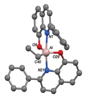
Fig. 5 The crystal structure of Al-E. Selected bond lengths (Å) and angles (°); Al-N1 2.1892(10), Al-O9 1.7989(9), Al-N21 2.1527(10), Al-O29 1.8007(10), Al-C40 1.9746(13), N1-Al-O9 82.28(4), N1-Al-N21 165.14(4), N1-Al-O29 89.27(4), N1-Al-C40 94.77(5), O9-Al-N21 88.62(4), O9-Al-O29 109.02(5), O9-Al-C40 122.89(5), N21-Al-O29 82.59(4), N21-Al-C40 100.04(5), O29-Al-C40 128.02(5).
