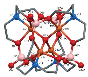
Fig. 5 The crystal structure of 4. H-atoms omitted for clarity, selected bond lengths (Å), Cu(1)-O(23) 1.9253(15), Cu(1)-N(1) 2.000(2), Cu(1)-O(4) 2.029(4) Cu(1)-O(10) 2.031(4), B(1)-O(4) 1.510(5), B(1)-O(4') 1.437(6).
