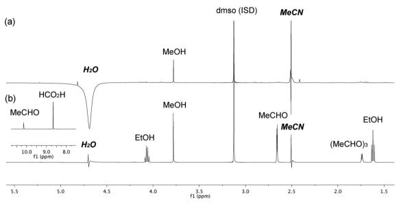
Fig. 6 (a) Liquid phase analytes from the oxidation of methane catalysed by 4. (b) Double solvent-suppression NMR method for the quantification of liquid-phase analytes of methane oxidation, inset is the downfield region showing the deshielded resonances of MeCHO and HCO<sub>2</sub>H.
