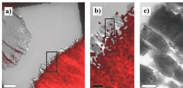
Fig. 32 (a) Fluorescence microscopy/TEM overlay image of a brightly fluorescing FCC particle slice. (b) Zoom-in of (a) in which the black rectangle shows the periphery of the particle, which is not fluorescent. (c) TEM imaging of the area boxed in (b) confirming the presence of a rim of clotted zeolites surrounding this FCC catalyst particle. (Reproduced with permission from ref. 183, Copyright Wiley-VCH, 2013).
