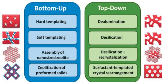
Fig. 18 Bottom-up and top-down approaches to hierarchical mesoporous zeolites. (Reproduced with permission from ref. 83, Copyright Wiley-VCH, 2014.)
