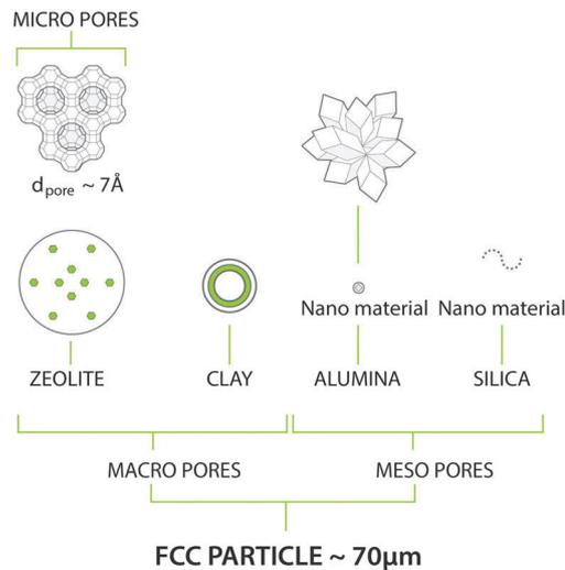
Fig. 7 Typical chemical and structural composition of a FCC particle. Artwork by RSK Communication.
