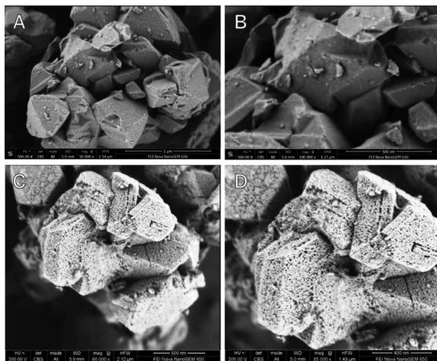
Fig. 19 FE-SEM images from untreated (top) and mesostructured (bottom) zeolite Y crystals. Scale bars: (a) 1  $\mu\text{m}$ ; (b and c) 500 nm; (d) 200 nm. (Reproduced with permission from ref. 83, Copyright Wiley-VCH, 2014).
