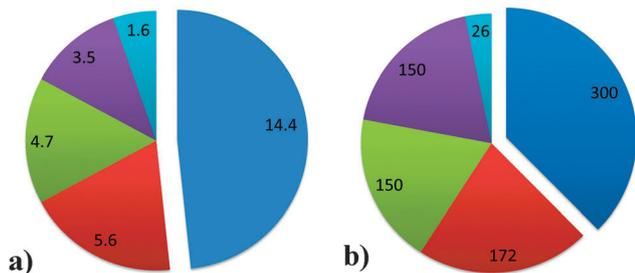
**Fig. 1** (a) Installed capacities for the major conversion processes in refineries worldwide, in million barrels per day. (b) Number of refineries in which major conversion processes are installed. Refineries can have more than one technology installed. Data as of 2013, from ref. 1. Color-coding: fluid catalytic cracking (FCC): blue; hydrocracking: red; coking: green; thermal operations: purple; and resid hydrotreating: light blue.
