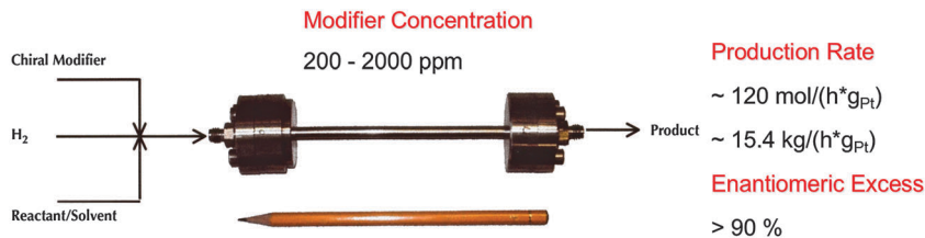
Fig. 9 Process intensification by continuous reactor operation mode.
