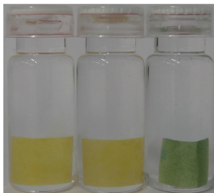
Fig. 7 Samples of Ethaline (left) Glyceline (middle) and Reline (right) with 20 wt% water and each containing a sample of universal indicator paper.
