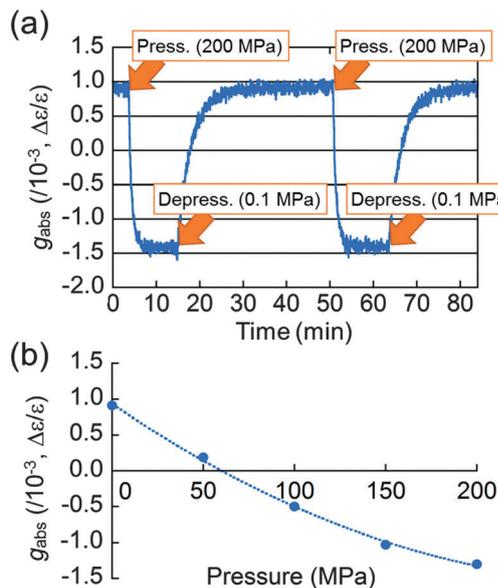
Fig. 2 (a) Time-resolved CD intensity change of **1** in 1,2-DCE at 368.0 nm exposed to pressurization (200 MPa) and depressurization (0.1 MPa) cycles. (b) Correlation between pressure and  $g_{\text{abs}}$  of **1** in 1,2-DCE at 368.0 nm.
