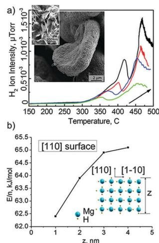
**Fig. 1** (a) Temperature programmed desorption of hydrogen from the sonogenerated metal-hydrogen sponge for reactive hard templating (sono-RHT); arrows show a ramping rate increase from 5 K min<sup>-1</sup> to 20 K min<sup>-1</sup> with the 5 K min<sup>-1</sup> step. Insets show SEM and TEM images of sono-RHT. (b) Normalized per number of Mg-atoms desorption energies of hydrogen of different thickness slabs within the DFT level.
