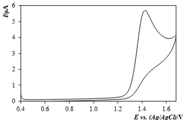
Fig. 2 Cyclic voltammogram of methiocarb (MTC) in solution  $0.1 \text{ mol L}^{-1} \text{ H}_2\text{SO}_4 + \text{MeOH}$  (10%, v/v) exp. conditions: CV,  $E_{\text{in}} +0.4 \text{ V}$ ,  $E_{\text{fin}} +1.7 \text{ V}$  vs. ref., scan rate:  $40 \text{ mV s}^{-1}$ ,  $c_{\text{MTC}} = 9.8 \text{ mg mL}^{-1}$ .
