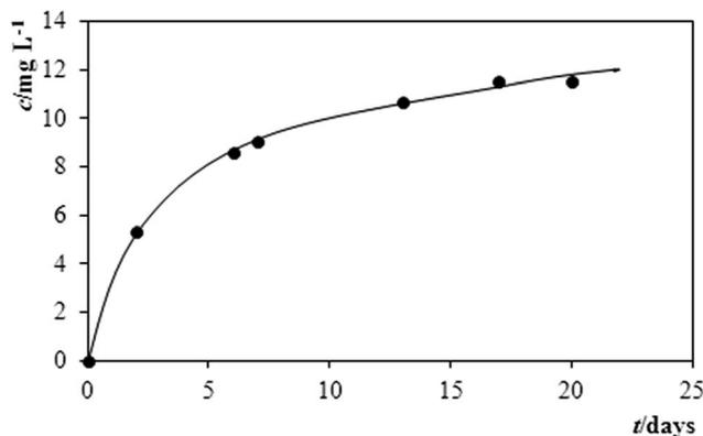
Fig. 5 Monitoring the activity of MTC in Mesurol via the time dependence of its gradually increasing solubility in model solution made of pond water.
