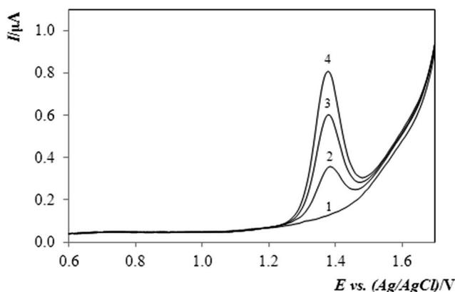
Fig. 3 DP-voltammograms of MTC in the supporting electrolyte ( $0.1 \text{ mol L}^{-1} \text{ H}_2\text{SO}_4$  in MeOH (10%, v/v)). Exp. conditions: DPV,  $E_{\text{in}} +0.4 \text{ V}$ ,  $E_{\text{fin}} +1.85 \text{ V}$ , scan rate:  $40 \text{ mV s}^{-1}$ , curve (1) supporting electrolyte, (2) MTC in model sample ( $c = 2.94 \text{ μg mL}^{-1}$ ), (3 and 4) additions of a  $30 \text{ μL}$  MTC standard solution ( $c_{\text{MTC}} = 0.98 \text{ mg mL}^{-1}$ ).
