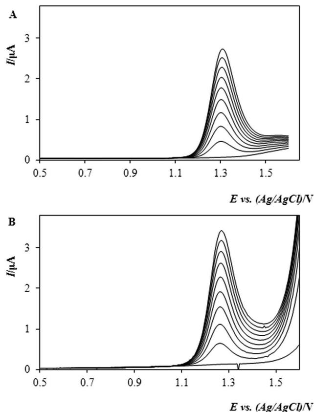
Fig. 1 DP-voltammograms of MTC in the supporting electrolyte of (A) 0.1  $\text{mol L}^{-1}$   $\text{H}_2\text{SO}_4$  and (B) 0.1  $\text{mol L}^{-1}$  citrate buffer with pH 6.62. Exp. conditions: DPV ramp,  $E_{\text{in}}$  +0.3 V,  $E_{\text{fin}}$  +1.6 V, scan rate: 40  $\text{mV s}^{-1}$ , MTC in the concentration range of 9.7  $\mu\text{g mL}^{-1}$  to 80.9  $\mu\text{g mL}^{-1}$ .
