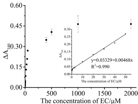
Fig. 2 The relationship between the change in absorbance at 340 nm and the concentration of EC. The inset shows the derived linear relationship and regression equation. The reaction time is 5 min.
