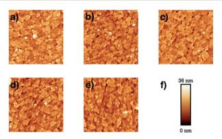
Fig. 3 Atomic force microscopy topography images of ZnO NP thin films corresponding to the following annealing conditions: (a) non-annealed, (b) 120 °C, (c) 150 °C, (d) 180 °C and (e) 210 °C. The area scanned for each image was 5  $\times$  5  $\mu m$  and (f) the  $\emph{Z}$ -scale for each image is also identical.
