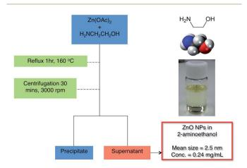
Scheme 1 Synthesis and separation of ZnO nanoparticles.
