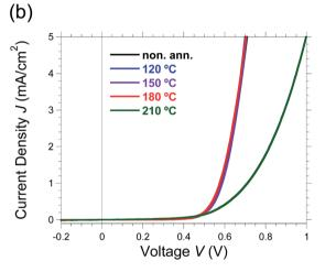
**Fig. 2** J-V curves for inverted P3HT:mix-PCBM devices where the ZnO NP film was subject to various annealing temperatures measured under (a) 1 Sun illumination (AM 1.5 G, 100 mW cm $^{-2}$ ) and (b) dark conditions. Non-annealed (black), 120 °C (blue), 150 °C (purple), 180 °C (red) and 210 °C (green).
