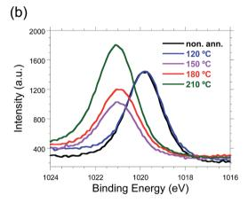
Fig. 4 X-ray photoelectron spectroscopy spectra of ZnO films corresponding to (a) N 1s and (b) Zn 2p<sub>3/2</sub> under the following annealing conditions: non-annealed (black), 120 °C (blue), 150 °C (purple), 180 °C (red) and 210 °C (green).
