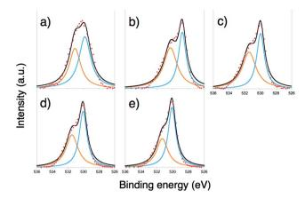
Fig. 5 XPS spectra of the O 1s peaks of the ZnO films under the following annealing conditions: (a) non-annealed, (b) 120 °C, (c) 150 °C, (d) 180 °C and (e) 210 °C. The orange and blue fits correspond to the deconvoluted O<sup>2-</sup> species, the former being an oxygen deficient species and the latter peak consistent with that of  $O^{2-}$  in a perfect wurtzite crystal. The raw data are represented by red circles along with best fits shown as a black line.
