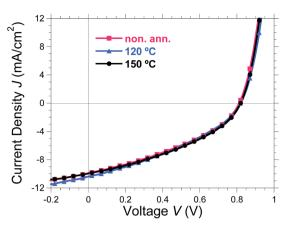
Fig. 6 J-V curves under 1 Sun illumination (AM 1.5 G, 100 mW cm $^{-2}$ ) for inverted SQ:PC<sub>71</sub>BM devices where the ZnO NP film was annealed at 120 °C (blue, triangles) and 150 °C (black, circles) as well as non-annealed (pink, squares).
