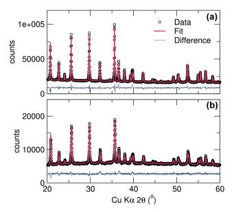
Fig. 4 Rietveld analysis was performed on single phase materials (a) LFP\_EG2 [ $R_{\rm wp}$  14.8%,  $R_{\rm exp}$  4.15%, a = 10.327 Å, b = 5.999 Å, c = 4.697 Å] and (b) LFP\_IL [ $R_{\rm wp}$  14.3%,  $R_{\rm exp}$  8.12%, a = 10.327 Å, b = 6.003 Å and c = 4.693 Å].
