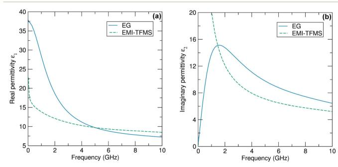
Fig. 1 (a) Experimental data for the real part  $\varepsilon_1$  of the complex permittivity  $\varepsilon$  measured as a function of frequency for the polar liquid ethylene glycol (EG) and the ionic liquid EMI-TFMS. (b) The same plot, only this time for the imaginary part  $\varepsilon_2$ . No errors bars are shown but all data are subject to a systematic error of  $\pm 1\%$  imposed by the aperture module of the coaxial probe used to extract the permittivity data.<sup>41</sup>
