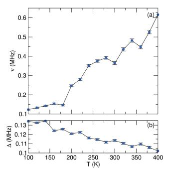
Fig. 8 Temperature dependence of (a) fluctuation rate ( $\nu$ ) and (b) field distribution width ( $\Delta$ ) parameters derived from fitting  $\mu$ SR data to a dynamic Kubo-Toyabe function for the LFP\_EG1 sample, measured from 100 K to 400 K.
