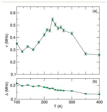
Fig. 7 Temperature dependence of (a) fluctuation rate ( $\nu$ ) and (b) field distribution width ( $\Delta$ ) parameters derived from fitting  $\mu$ SR data to a dynamic Kubo-Toyabe function for the LFP\_IL sample, measured from 100 K to 400 K.
