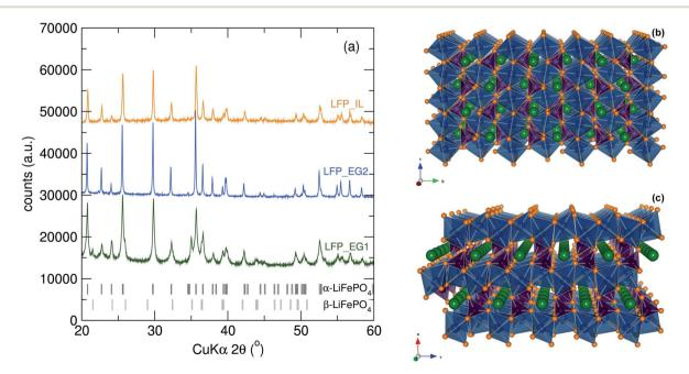
Fig. 3 (a) XRD data for LFP\_EG1 reveals this is a two-phase system, comprising the *Pnma* structured LiFePO<sub>4</sub>) and the high pressure Cmcm phase (β-LiFePO<sub>4</sub>). These phases are depicted in (b) Cmcm high pressure LiFePO<sub>4</sub> and (c) Pnma LiFePO<sub>4</sub>.
