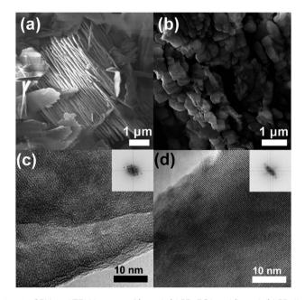
**Fig. 5** SEM and TEM images of (a and c) LFP\_EG1 and (b and d) LFP\_IL, respectively. Large, stacked platelets and rods, with a typical thickness of 20 nm are noted for the EG1 sample, while more crystalline particles are seen for the IL sample. Long-range crystallinity throughout particles of both samples was confirmed by HRTEM images, with (inset) Fourier transforms demonstrating long-range crystallographic ordering (c and d).
