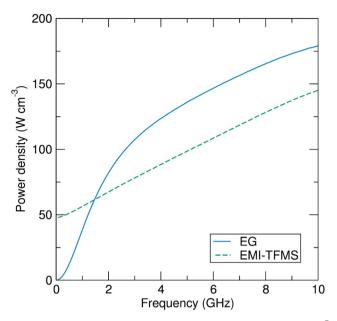
Fig. 2 The rms dissipated power density P (expressed in W cm $^{-3}$ ) calculated from the permittivity data of Fig. 1 for a uniform internal electric field of magnitude 10 kV m<sup>-1</sup>, plotted as a function of frequency
