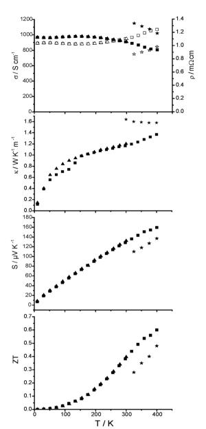
Fig. 9 Thermoelectric properties of (GeTe)<sub>5.5</sub>AgInTe<sub>2</sub> (heating curve: ■; cooling curve: ▲), from top to bottom: electrical conductivity and resistivity (solid and empty symbols, respectively), thermal conductivity, Seebeck coefficient and *ZT* value in comparison to values for TAGS-85 (asterisks) taken from ref. 19.
