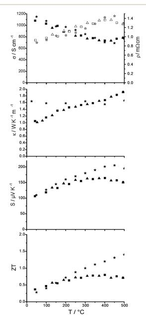
Fig. 8 Thermoelectric properties of (GeTe)<sub>5.5</sub>AgIn<sub>0.5</sub>Sb<sub>0.5</sub>Te<sub>2</sub> (heating curves: ■; cooling curves: ▲), from top to bottom: electrical conductivity and resistivity (solid and empty symbols, respectively), thermal conductivity, Seebeck coefficient and ZT value in comparison to values for TAGS-85 (asterisks) taken from ref. 19
