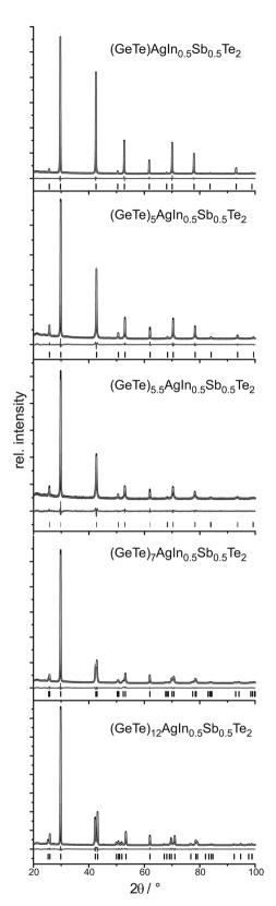
Fig. 2 Rietveld fits for  $(GeTe)_x AgIn_{0.5} Sb_{0.5} Te_2$  (x = 1, 5, 5.5, 7 and 12; from top to bottom – HP synthesis for x = 1): experimental (black) and calculated data (gray); difference plot (gray, below); and peak positions (black, vertical lines).
