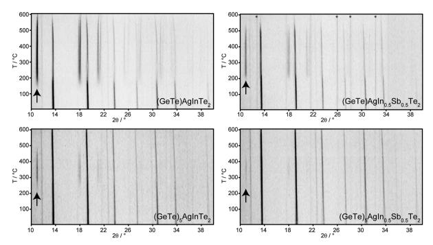
Fig. 6 Temperature-dependent X-ray powder diffraction patterns of  $(GeTe)_x AgIn_y Sb_{1-y} Te_2$  for x=1 (top) and 5 (bottom); y=1 (left) and 0.5 (right); asterisks (\*) mark reflections caused by the furnace; the arrows mark the strongest reflection of AgInTe<sub>2</sub>.
