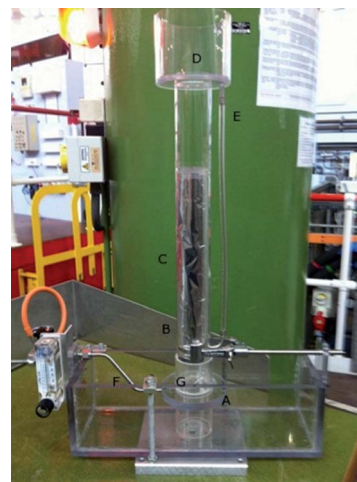
Scheme 1 SANS sample environment for studying foams.
