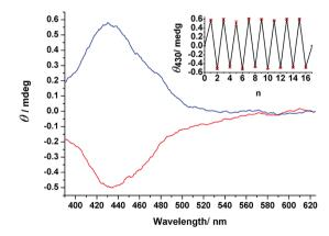
Fig. 6 Induced CD spectra of an MeCN solution of 3 upon irradiation with r-CPL (blue line) and I-CPL (red line) at 436 nm. Inset: CD intensities at 430 nm for a solution of 3 upon alternating irradiation with r- and l-CPL (n = 1-16) and non-polarized light (n = 17), with a standard error of mean values from three independent experiments. Because the concentration was too high (1.33 imes  $10^{-3}$  M), it was impossible to measure the CD spectra at wavelengths of less than 390 nm.
