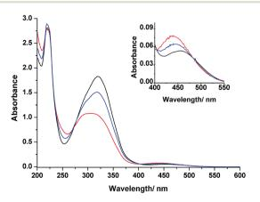
Fig. 3 UV-Vis spectra of MeCN solution of 3 (4.69  $\times$  10<sup>-4</sup> mol L<sup>-1</sup>) at room temperature: (a) initial state prior to irradiation (black line); (b) PSS<sub>366 nm</sub> (red line); (c) PSS<sub>436 nm</sub> (blue line). Inset: enlarged view of the  $n-\pi^*$  band.
