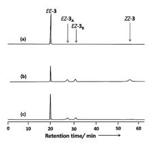
Fig. 4 Chiral HPLC chromatograms (solvent: isopropanol/hexane, 1:4; flow rate:  $1\,\text{mL min}^{-1}$ ) of **3**: (a) before irradiation; (b) the PSS after irradiation at 366 nm; (c) the PSS after irradiation at 436 nm.
