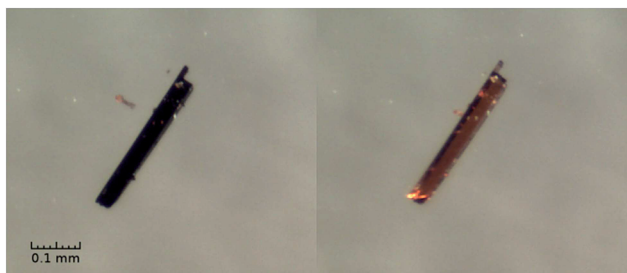
Fig. 4 Light microscope image of SC-to-SC deoxygenation of [(\text{bpbp})\text{Co}_2(\text{O}_2)_2(\text{NH}_2\text{bdc})](\text{NO}_3)_4 \cdot 7\text{H}_2\text{O} , ( 2b (NO 3 ) 4 ·7H 2 O) (left) to give [(\text{bpbp})\text{Co}_2(\text{NO}_3)_2(\text{NH}_2\text{bdc})](\text{NO}_3)_2 \cdot 2\text{H}_2\text{O} , 2b deoxy (NO 3 ) 2 ·2H 2 O (right). Transformation performed by heating for approximately 5 minutes on a regular hot-plate set to a temperature of 80 °C.
