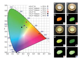
Fig. 7 Chromaticity diagram and photographs of LaPO<sub>4</sub>:Eu<sup>3+</sup> 10% (a and b), LaPO<sub>4</sub>:Eu<sup>3+</sup> 10%@organic (c–e), LaPO<sub>4</sub>:Tb<sup>3+</sup> 10% (f and g) and LaPO<sub>4</sub>:Tb<sup>3+</sup> 10%@organic (h–j), taken in daylight (a, c, f and h) and under UV light irradiation ( $\lambda_{ex} = 210$  nm – g and i;  $\lambda_{ex} = 250$  nm – b and d;  $\lambda_{ex} = 300$  nm – e and j).
