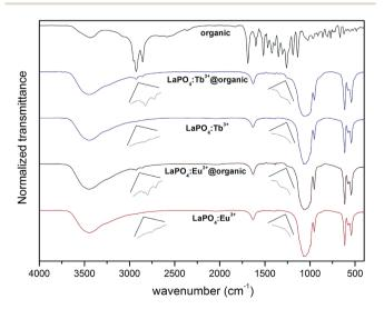
Fig. 4 IR spectra of pure organic compound (surface modifier), unmodified LaPO<sub>4</sub>:Eu<sup>3+</sup> 10% and LaPO<sub>4</sub>:Tb<sup>3+</sup> 10%, surface modified LaPO<sub>4</sub>:Eu<sup>3+</sup> 10%@organic and LaPO<sub>4</sub>:Tb<sup>3+</sup> 10%@organic.
