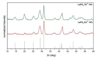
Fig. 2 XRD patterns of LaPO<sub>4</sub>:Eu<sup>3+</sup> 10% (0.5H<sub>2</sub>O) and LaPO<sub>4</sub>:Tb<sup>3+</sup> 10%  $(0.5H_2O)$
