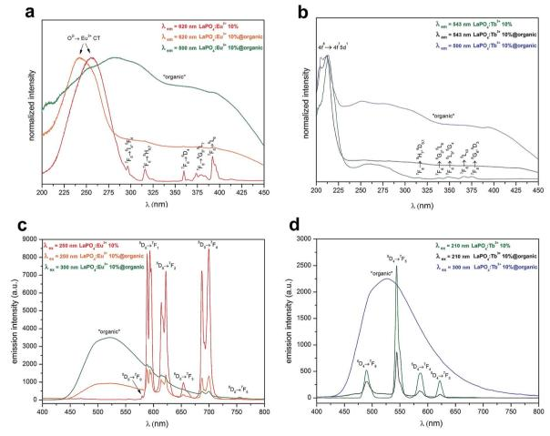
Fig. 6 Excitation spectra of LaPO $_4$ :Eu $^{3+}$  10%, LaPO $_4$ :Eu $^{3+}$  10%@organic (a) and LaPO $_4$ :Tb $^{3+}$  10%, LaPO $_4$ :Tb $^{3+}$  10%@organic (b); emission spectra of LaPO $_4$ :Eu $^{3+}$  10%, LaPO $_4$ :Eu $^{3+}$  10%@organic (c) and LaPO $_4$ :Tb $^{3+}$  10%@organic (d).
