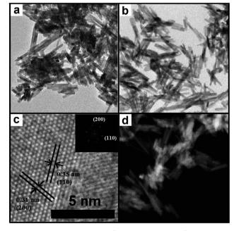
Fig. 3 TEM images of LaPO<sub>4</sub>:Eu<sup>3+</sup> 10% (a), LaPO<sub>4</sub>:Tb<sup>3+</sup> 10% (b); HR-TEM image and its FFT inset for LaPO<sub>4</sub>:Eu<sup>3+</sup> 10% (c); STEM image of LaPO<sub>4</sub>:Eu<sup>3+</sup> 10% (d).
