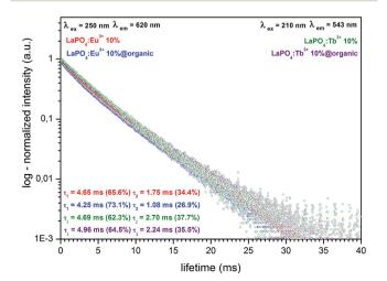
Fig. 8 Luminescence decay curves of LaPO $_4$ :Eu $^{3+}$  10%, LaPO $_4$ :Eu $^{3+}$  10%@organic and LaPO $_4$ :Tb $^{3+}$  10%, LaPO $_4$ :Tb $^{3+}$  10%@organic.
