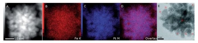
Fig. 1 STEM-HAADF images and elemental mapping of sample 14, mcNPs prepared in dioctyl ether with 4.5 mmol (17%) OA and tSf equal to 31.5 mmol; A, STEM-HAADF, B, Fe distribution; C, Pt distribution; D, overlay of Fe and Pt layers; E, HRTEM.
