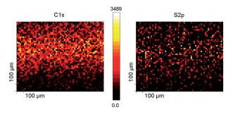
Fig. 4 XPS mapping plots of the Au<sup>TS</sup>- $\beta$ CDSAM//G1-PPI-(Fc)<sub>4</sub> surface of the elements C1s and S2p on an area that had been in contact with the top-electrode (the contact area of 300  $\mu$ m<sup>2</sup> is approximately in the middle of the image of 100  $\times$  100  $\mu$ m<sup>2</sup>), but the surrounding area not. See text for details.
