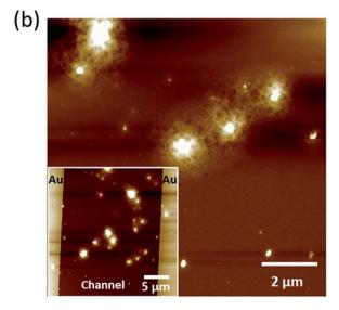
Fig. 7 AFM images scanned inside the channel of films of: (a) pristine P3HT and (b) 24% GNR with P3HT. The insets show the scan at a larger scale. Z-scales: (a) 17 nm, (b) 75 nm, inset (a) 47 nm, inset (b) 92 nm.
