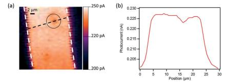
Fig. 10 (a) Zero drain bias photocurrent response for OFET with 24% GNR/P3HT and  $L=20~\mu m$  in the off-state ( $V_G=+30~V$ ). The dashed white lines indicate the edges of the source and drain electrical contacts; the black circle indicates the observed aggregate of GNRs. (b) Variation of the photocurrent as a function of the position of the black dashed line in (a).
