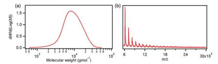
Fig. 2 (a) Molecular weight distribution of polyphenylene precursor 6 (SEC analysis, eluent: THF, polystyrene standard). (b) Linear-mode MALDI-TOF MS spectrum of polyphenylene precursor 6.
