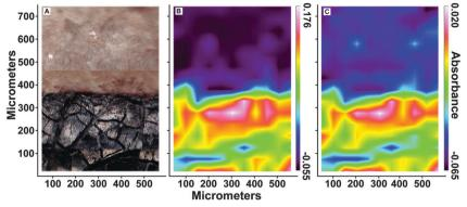
Fig. 5 (A) Optical microscope image of fossilized leaf material [stem, bottom] and sedimentary matrix [top]. Infrared absorption maps of same area at (B) 1560 cm<sup>-1</sup> and (C) 2930 cm<sup>-1</sup> in leaf material (attenuated total reflectance mode). Absorbance is scaled from low (purple) to high (red/white). These maps show that organic functional groups are highly constrained within the fossil residue.
