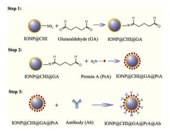
Fig. 1 Step 1: Glutaraldehyde (GA) chitosan was conjugated to chitosan-coated IONP (IONP@CHI) and step 2: reaction of IONP@CHI@GA and protein A (PrA) to form the conjugate of IONP@CHI@GA@PrA. Step 3: preparation of IONP@CHI@GA@PrA linked with specific antibodies against pathogens via their bio-affinity.
