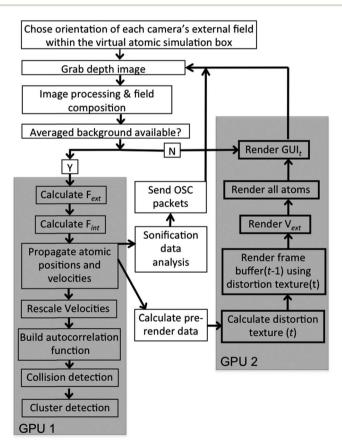
Fig. 3 Flow chart showing system operation. The grey blocks indicate those portions of the system that we accelerated on GPUs; the remaining functionality is executed on the CPU.
