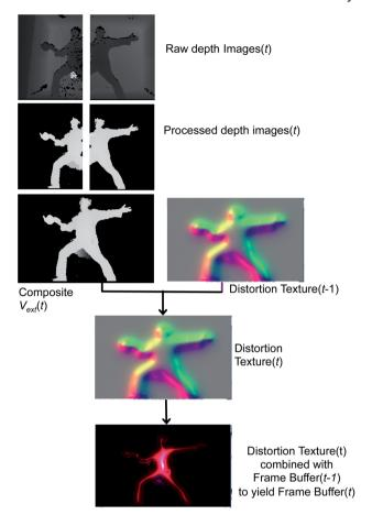
Fig. 5 Pipeline showing how graphics rendering is done in dS. The figure shows how images from two depth sensors are combined to yield  $V_{\rm ext}$ , the distortion texture, and the final frame buffer. An example of the final frame buffer is shown, with only  $V_{\rm ext}$  and no atoms.
