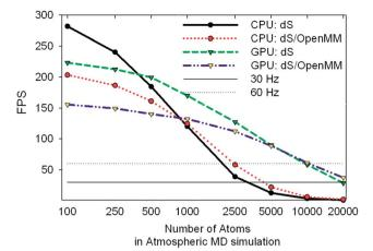
Fig. 8 Benchmark data showing frames per second obtained for the same tests described in Fig. 7. The 30 and 60 Hz limits are shown for reference.
