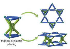
Fig. 43 Schematic showing the possible axial-to-axial (A-A) pillaring of kgm layers by trigonal prism pillars, leading to lon-e topology.
