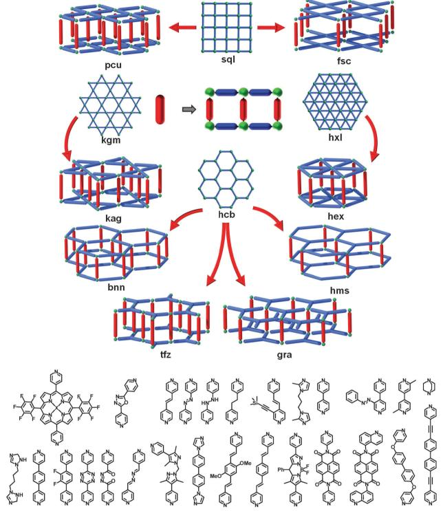
Fig. 28 Schematic of the A–A pillaring of sql, kgm, hxl, and hcb layers to form the pcu, fsc, kag, hex, bnn, hms, gra, and tfz nets (top), and a non-exhaustive list of ligands that have been used for this type of pillaring (bottom).
