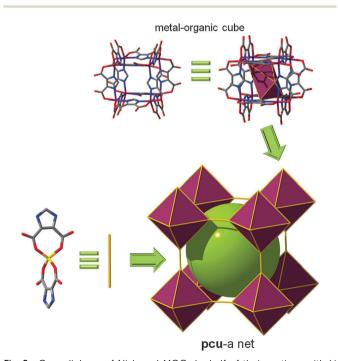
Fig. 9 Cross-linkage of Ni-based MOCs by half of their vertices with Li leads to a MOF with underlying pcu topology, where the MOC is 6-c, forming an octahedral SBB.
