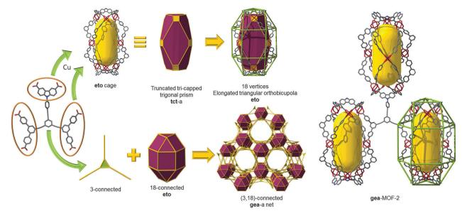
Fig. 26 Schematic showing the design path followed to achieve the construction of gea-MOF-2, the first SBB-based gea-MOF
