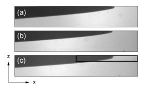
Fig. 4 Images of the reaction front in a closed reactor at  $g_z/g_0 = 1.0$  (a), 1.7 (b) and 0.01 (c). The black rectangle in (c) is the window where the front evolution of the tip was monitored to construct Fig. 5. Field of view: 5.8 cm  $\times$  1.0 cm.
