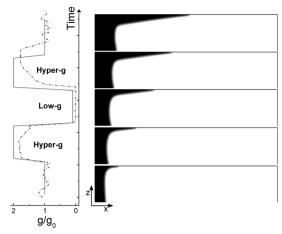
Same as in Fig. 8 but when only Marangoni effects are operative (Ra = 0, Ma = 10). The front propagates at a constant speed and is unaffected by changes in the amplitude of gravity. No return flow is observed at the surface.
