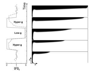
Fig. 10 Same as in Fig. 8 but when the hydrodynamic flows are driven by the cooperative contribution of buoyancy and Marangoni effects (Ra = 0.2, Ma = 10). The dynamics are a combination of those of Fig. 8 and 9, i.e. a slowing down of the buoyancy effect is obtained in the micro-gravity phase but no return flow is obtained as in the Marangoni-driven flow field.
