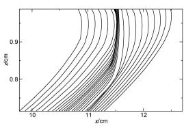
Fig. 5 Spatio-temporal evolution of front profiles with  $\Delta t=2$  s for a reaction front propagating from left to right in a closed cell within the black window shown in Fig. 4(c) as the plane enters the micro-g phase from the hyper-g phase and back again.
