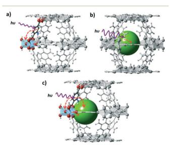
Fig. 3 Different approaches to induce photocatalytic activity in a MOF scaffold: a) the organic linker is used as an antenna for light sensitizing and charge transfer to the inorganic cluster occurs; b) the MOF is used as a container for the encapsulation of a photocatalyst that directly absorbs light and c) charge transfer occurs between the MOF scaffold and the encapsulated catalyst.
