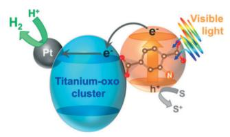
Fig. 4 A schematic illustration of photocatalytic hydrogen production reaction over Pt-supported Ti-MOF-NH2 on the basis of the LCCT mechanism.<sup>60</sup> Reproduced with permission from the American Chemical Society.
