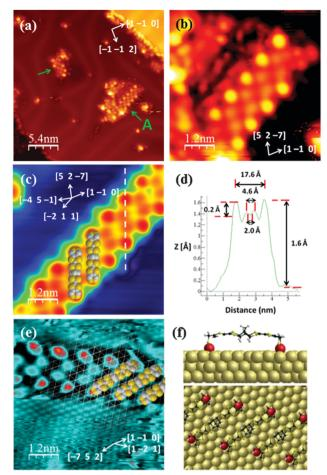
Fig. 3 STM images of TAT-TTF islands on Au(111) after annealing to 333 K (a) -0.6 V, 0.06 nA,  $27 \times 27$  nm<sup>2</sup>; (b) Island A, -0.6 V, 0.06 nA,  $6 \times 6$  nm<sup>2</sup>; (c) -0.9 V, 0.08 nA,  $6 \times 6$  nm<sup>2</sup>; (d) Line profile taken along white line indicated in (c); (e) -0.2 V, 0.13 nA,  $6 \times 6$  nm<sup>2</sup>; (f) Optimised DFT geometry of TAT-TTF bound *via* gold adatoms (red) to surface atoms (dark yellow).
