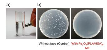
Fig. 5 (a) Photograph of collection of *E. coli*-loaded  $Fe_3O_4(PLA/HSA)_9$  MTs by a magnetic field. (b) Appearance of LB agar plates spread with *E. coli* dispersion which was incubated with  $Fe_3O_4(PLA/HSA)_9$  MTs for 30 min (after 16 h cell culture at 37 °C).
