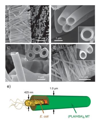
Fig. 1 SEM images of (PLA/HSA)<sub>9</sub> MTs prepared using a porous PC template ( $D_p = 1.2 \mu m$ ): (a, b) dried samples and (c) lyophilized sample after swelling in water. (d) SEM image of Fe<sub>3</sub>O<sub>4</sub>(PLA/HSA)<sub>9</sub> MTs prepared using a porous PC template ( $D_p = 1.2 \mu m$ ). (e) Schematic illustration of E. coli entrapped (PLA/HSA)<sub>9</sub> MTs.
