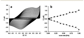
Fig. 1 (a) Cyclic voltammograms of CoP-ssDNA on the Au-electrode at scan rates from 10 to 1000 mV s $^{-1}$ ; buffer conditions: 1.0 M NaCl, 0.01 M sodium citrate, pH 7.0; (b) plots of anodic (♠) and cathodic (■) current vs.
