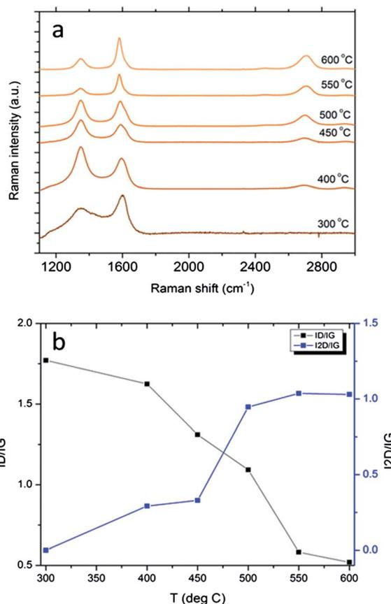
Fig. 6 (a) Raman spectra of graphene products grown at different temperatures by CVD on nickel foils with acetylene as a carbon source. (b)  $I_D/I_G$  (black) and  $I_{2D}/I_G$  (blue) intensity ratios versus growth temperature.
