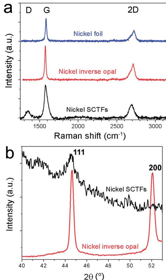
Fig. 4 (a) Raman spectra of graphene grown from methane at 1000 °C on a nickel foil (blue), inverse opals (red) and SCTFs (black). (b) XRD spectra of nickel inverse opals (red) and nickel SCTFs scaled  $\times 100$  (black).
