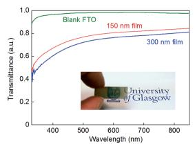
Fig. 4 UV-vis transmission spectra of a 300 nm-thick Co-doped molybdenum sulfide film on FTO (blue line), a 150 nm-thick Co-doped molybdenum sulfide film on FTO (red line), and a blank FTO substrate for comparison (green line). A 1 mm-thick solid metal plate had a transmittance of zero on this scale (data not shown). Inset: a photograph of a 150 nm-thick Co-doped molybdenum sulfide film on FTO showing its translucent nature.
