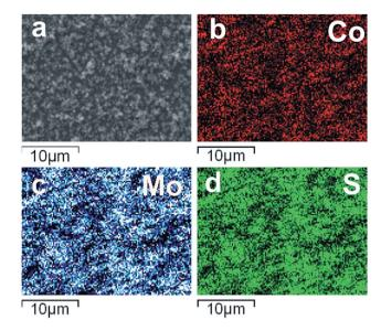
Fig. 3 SEM images and the corresponding elemental mapping for Co, Mo and S in a Co<sub>2</sub>Mo<sub>9</sub>S<sub>26</sub> film, indicating the homogeneous distribution of Co atoms within the sample.
