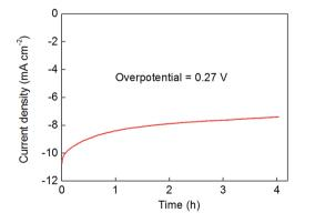
Fig. 6 Controlled potential bulk electrolysis of a 300 nm-thick Co<sub>2</sub>Mo<sub>9</sub>S<sub>26</sub> film on an FTO support at a fixed, resistance-corrected overpotential for the hydrogen evolution reaction of 270 mV. The electrolyte was 0.5 M H<sub>2</sub>SO<sub>4</sub> and was stirred throughout (see Experimental section for further details).
