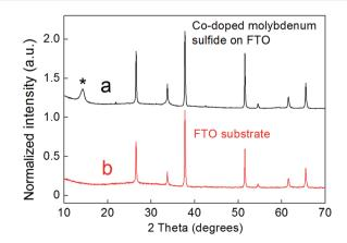
Fig. 1 (a) XRD pattern of a Co-doped molybdenum sulfide film grown on an FTO substrate (black). The peak associated with the hexagonal structure of MoS<sub>2</sub> is highlighted with the asterisk. (b) The XRD pattern of a blank FTO substrate for comparison (red).
