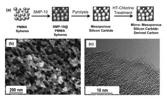
Fig. 1 Schematic of the synthesis procedure (a), SEM micrograph (b), and TEM micrograph (c) of hierarchical CDC from sacrificial PMMA
