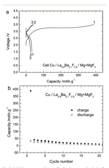
Fig. 9 (a) Voltage-composition profiles for the same cell with the Cu cathode vs. the Mg + MgF<sub>2</sub> anode in the three first cycles and (b) Cycling behaviour of this cell during 20 cycles. The charge/discharge curves were obtained at 150 °C for a current density of ca. ±4 mA g
