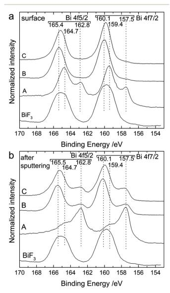
Fig. 8 XP spectra of the Bi 4f region measured at (a) the surface and (b) after sputtering the outer layer of the back side of the cathode for a Bi/  $La_{0.9}Ba_{0.1}F_{2.9}/Mg + MgF_2$  cell after cell preparation (as-milled cathode) (A), after charging to 3.2 V (B) and after discharge (C). For comparison, the intensities of all spectra were normalised to 1.
