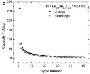
Fig. 6 (a) Voltage-composition profiles for a cell with the Bi cathode vs. Mg + MgF<sub>2</sub> anode in the three first cycles and (b) cycling behaviour of this cell during 50 cycles. The charge/discharge curves were obtained at 150 °C for a current density of ca.  $\pm 4$  mA g<sup>-1</sup>.
