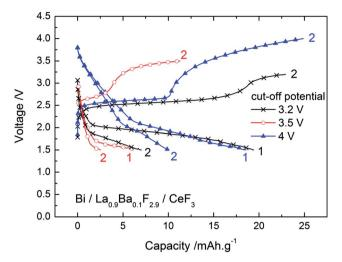
Fig. 3 Voltage-composition profiles for the Bi/La<sub>0.9</sub>Ba<sub>0.1</sub>F<sub>2.9</sub>/CeF<sub>3</sub> cell in the two first cycles (1st charges are given in Fig. S3, see ESI†). The charge/discharge curves were obtained at 150 °C for a current density of ca.  $\pm 4$  mA g<sup>-1</sup>
