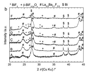
Fig. 1 (a) First charging curve obtained for a cell composed of a Bi cathode and CeF3 as the anode. The charging curve was obtained at 150 °C for a current density of ca. 4 mA  $g^{-1}$  and (b) XRD patterns measured after charging to different voltages: (A) before charging and after charging to (B) 2 V, (C) 2.5 V, (D) 3.2 V, (E) 4 V as indicated in the voltage profile and (F) after 1 cycle (charge + discharge).
