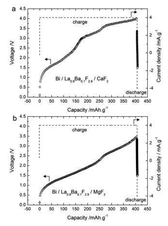
Fig. 4 Voltage-composition profiles for the first cycle of charging and discharging (150 °C,  $\pm 4$  mA g $^{-1}$ ) for the cells (a) Bi/La $_{0.9}$ Ba $_{0.1}$ F $_{2.9}$ /CaF $_{2}$ and (b) Bi/La<sub>0.9</sub>Ba<sub>0.1</sub>F<sub>2.9</sub>/MgF<sub>2</sub>. Symbols: voltage and dashed lines: current density.
