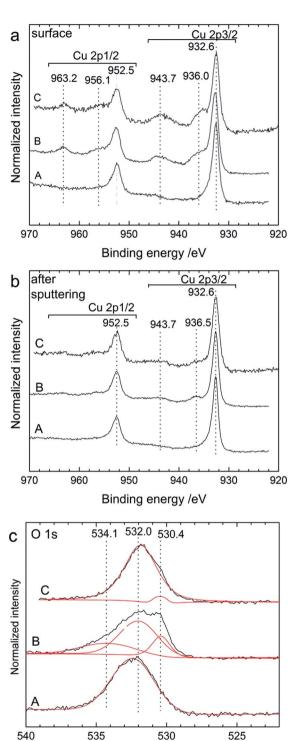
Fig. 11 XP spectra for the Cu 2p region measured at (a) the surface and (b) after sputtering the outer layer of the back side of the cathode and (c) XP spectra of the O 1s region (black: measurements and red: fit) after sputtering for a  $\text{Cu/La}_{0.9}\text{Ba}_{0.1}\text{F}_{2.9}/\text{Mg} + \text{MgF}_2$  cell after cell preparation (asmilled cathode) (A), after charging to 3.5 V (B) and after discharge (C). For comparison, the intensities of all spectra were normalised to 1.
