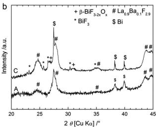
Fig. 5 XRD patterns of the cathode material after cycling a cell with Bi as the cathode to different stages, using (a) CaF2 as the anode or (b) MgF<sub>2</sub> as the anode. The patterns were recorded on the as-milled cathode composite (A), after charging to 3.2 V (B), after charging to 3.5 V (C), after charging to 4 V (D) and after one cycle (E)
