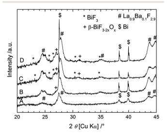
Fig. 7 XRD patterns measured on the back side of the cathode for a  $Bi/La_{0.9}Ba_{0.1}F_{2.9}/Mg + MgF_2$  cell before charging (A), after charging to 2.85 V (B), after charging to 3.2 V (C) and after discharge (D).
