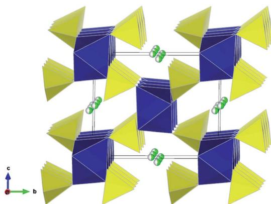
Fig. 2 Crystal structure of the delithiated phase  $\text{LiFe}(\text{SO}_4)_2$  showing  $\text{FeO}_6$  octahedra (blue),  $\text{SO}_4$  tetrahedra (yellow) and half occupied Li sites (green/white) running parallel to the  $a$ -axis. [Experimental refinement data in Table S2.†]
