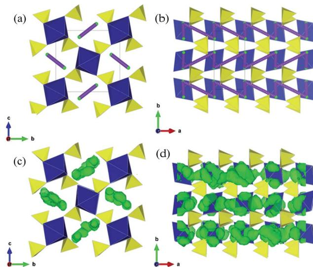
**Fig. 4** Low energy Li diffusion paths within [100] channels of  $\text{Li}_2\text{M}(\text{SO}_4)_2$  ( $\text{M} = \text{Fe}, \text{Mn}, \text{Co}$ ). (a) and (b) Static lattice calculations of low energy Li migration path combining L1 and L4 jumps. (c) and (d) Li density plots as calculated using MD at 473 K. (a), (c) and (b), (d) are equivalent views along the  $a$ -axis and  $c$ -axis respectively.
