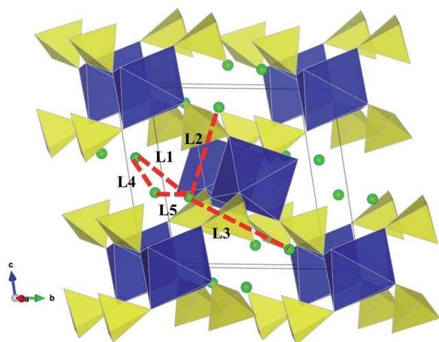
**Fig. 3** Lithium ion migration paths in  $\text{Li}_2\text{M}(\text{SO}_4)_2$  ( $\text{M} = \text{Fe}, \text{Mn}, \text{Co}$ ) between adjacent Li sites (with initial Li positions found in Table S2†). Li–Li jumps considered are labelled L1–L5 (with Li–Li separations found in Table S3†).
