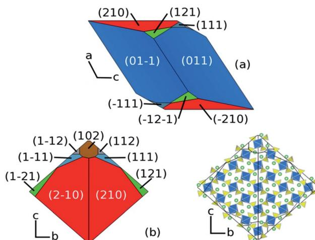
Fig. 5 Calculated particle morphology of  $\text{Li}_2\text{Fe}(\text{SO}_4)_2$ ; as viewed along (a) the *b*-axis, (b) the *a*-axis. In (c) the atomic structure is overlaid upon the *a*-axis view showing the availability of access to the 1D migration channels.
