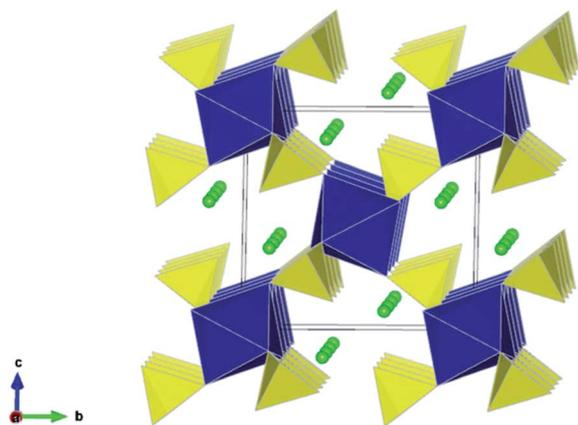
Fig. 1  $\text{Li}_2\text{M}(\text{SO}_4)_2$  ( $M = \text{Fe}, \text{Mn}, \text{Co}$ ) crystal structure showing  $\text{MO}_6$  octahedra (blue),  $\text{SO}_4$  tetrahedra (yellow) and chains of Li ions (green) running parallel to the  $a$ -axis. [Experimental refinement data in Table S2.†]
