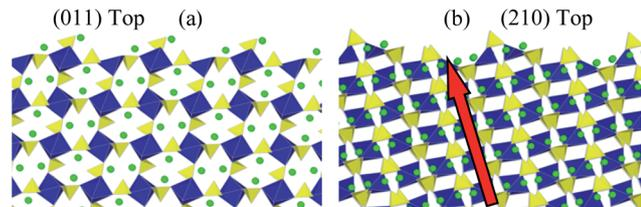
Fig. 6 Side view of relaxed (a) {011} and (b) {210} surfaces of  $\text{Li}_2\text{Fe}(\text{SO}_4)_2$ . The red arrow indicates the Li migration direction for {210} towards the outermost surface. For the {011} surface Li migration is into the page.
