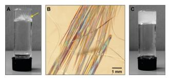
Fig. 5 (A) Digital photograph showing crystal growth in the gel made of 1 in 2-methylbutan-1-ol ( $c = 4.7 \text{ g L}^{-1}$ ) by heating-cooling. (B) Optical microscope picture of the crystals observed in (A). (C) Gradual crystal growth observed during the gelation of hexan-1-ol using **1** ( $c = 9.1 \text{ g L}^{-1}$ ) and the heating-cooling protocol. The gelator concentration corresponds to the CGC (Table 1).
