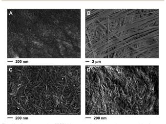
Fig. 11 Representative FESEM images of the xerogels prepared by freezedrying of the corresponding organogels made of  ${\bf 1}$  in different solvents at their CGC (Table 1). (A) Methanol (heating–cooling, c=7 g L $^{-1}$ ), (B) phenylmethanol (heating–ultrasound, c=21 g L $^{-1}$ ), (C) hexan-1-ol (heating–ultrasound, c=7 g L $^{-1}$ ) and (D) hexan-1-ol (heating–cooling, c=9.1 g L $^{-1}$ ). Note: the selected images are representative of the bulk material. For additional images see ESI.†
