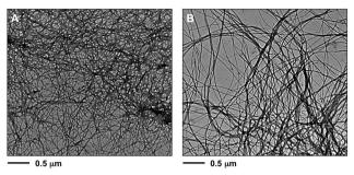
Fig. 12 Representative TEM images of xerogels of the corresponding organogels made of 1 in different solvents at the CGC (Table 1): (A) methanol (heating-cooling,  $c = 7 \text{ g L}^{-1}$ ), (B) hexan-1-ol (heatingultrasound,  $c = 7 \text{ g L}^{-1}$ ). Note: the selected images are representative of the bulk material. For additional images see ESI.†
