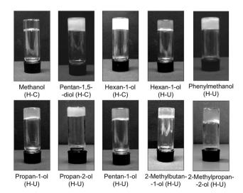
Fig. 2 Representative photographs of upside-down vials containing organogels made of gelator 1 in different alcohols prepared at the corresponding CGC (Table 1) via heating-cooling (H-C) or heating-ultrasound (H-U)
