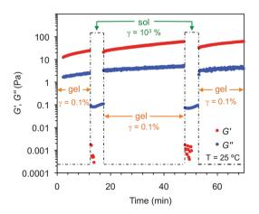
Fig. 15 Rheological loop test of the gel made of  $\mathbf{1}$  in butan-1-ol at CGC (c =8.4 g L<sup>-1</sup>). Steps: (1) 1 Hz, 0.1% strain, 10 min; (2) 0.1 Hz, 1000% strain, 5 min; (3) 1 Hz, 0.1% strain, 30 min. Steps 2 and 3 were repeated for a second cycle.
