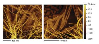
Fig. 13 Representative AFM images of the gel made of 1 in methanol (heating-cooling) at the CGC ( $c = 7 \text{ g L}^{-1}$ ). Note: the selected images are representative of the bulk material. For additional images see ESI.†
