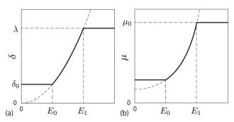
(a) Depletion length as a function of the applied electric field. (b) Electro-osmotic mobility as a function of the applied electric field.
