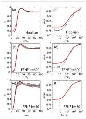
Fig. 6 (a) Concentration profiles of the Hookian dumbbell as a function of the distance from the surface. Points show the simulation results; the curved line is calculated by the kinetic theory. (b) Nonlinear electroosmotic mobilities of the Hookian dumbbell as a function of an applied electric field. (c) and (d) same as (a) and (b), respectively, but for the FENE dumbbell with b = 600. (e) and (f) Same as (a) and (b), respectively, but for the FENE dumbbell with b = 50
